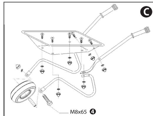
Screw the wheel onto the legs. Do not fully tighten the screws. Otherwise the wheel will not turn freely.
