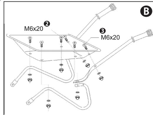
Screw the legs and handles onto the tub. Now fully tighten all the screws.
