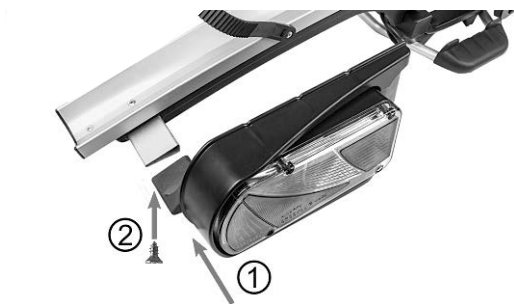
Figure 1: Installation of the rear lights
