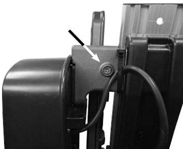
Figure 2: Installation of the rear lights
