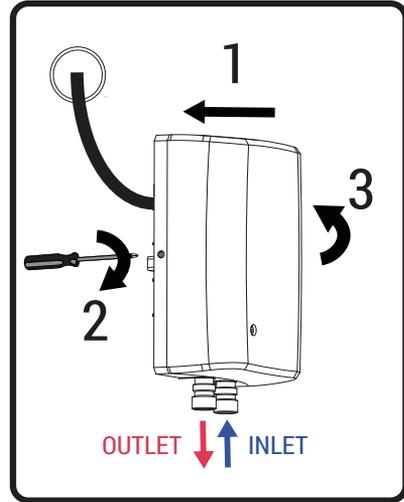
1. Switch off the power supply and prepare the mains cable as shown in B1 as shown.
