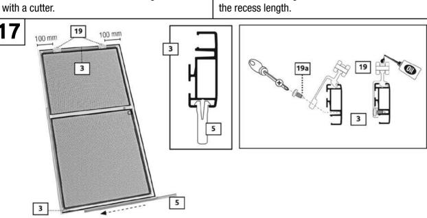
Attach both rollers **19** to the upper cross section **3** keeping 100 mm distance to the corners, by angling them as pictured 19a and attaching them using the four screws. If possible, oil the rollers. Insert the guide rail 5 into the groove of the lower section 3.
