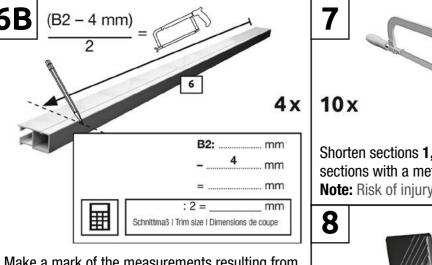
Make a mark of the measurements resulting from the following formulas on the four guide rails **6:** (B2 - 4 mm) / 2. To do so, deduct 4 mm from the determined jamb width B2 and divide the result by 2. Make a mark of this measurement on the sections. **Example:** Measured jamb width B2 = 1900 mm (1900 mm - 4 mm) / 2 = 948 mm.
