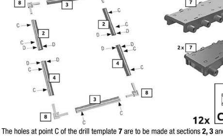
The holes at point C of the drill template 7 are to be made at sections 2, 3 and 4. Attach the drill template to both ends of the sections and drill from the outside with a 3.5 mm drill bit through the groove, which opens towards the side, towards the cavity of the section. Do NOT completely drill through the sections.
