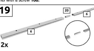
Attach both guide sections 6 in the middle with connectors 20.
