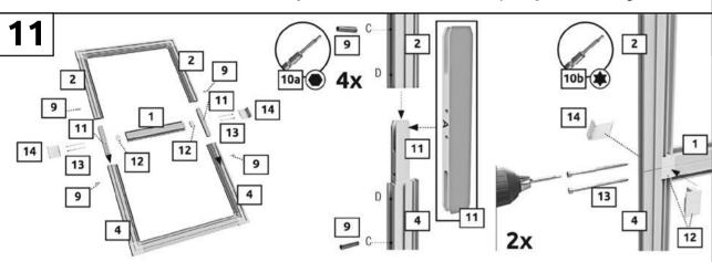
Insert the middle connector **11** half-way into section **4**, as pictured and attach with a threaded pin **9** in located on the sections. Screw sections 2 and 4 together with middle section 1 through both holes D using screws 13. Attach the covering caps 14 to the frame.
