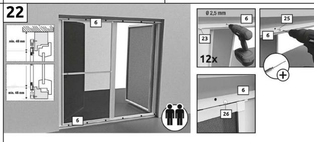
The door is ready to be attached to the door frame. The upper edge of the upper guide rail is located 48 mm above the doorway, the lower edge of the lower guide rail is located 48 mm below the doorway. Using a 2.5 mm drill, drill through the holes in guide profile 6 into the frame and screw together with screws 25. Take care that the door doesn't catch against guide profile 6, it must hang freely. Then push the covering caps 26 into the drill holes.
