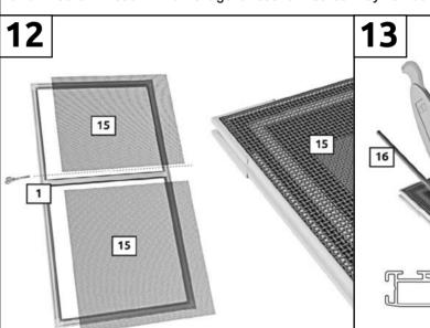
Attach the material 15 with a rubber welt 16 around the welt groove on the sections. Use the wide side A of the welt tool to do this **17.** Shorten the welt 16 with scissors after you have attached it all around.
