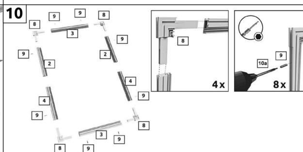
Connect both sections 2 to the upper with the upper cross section 3, and both sections 4 with the lower cross section 3, using corner connectors 8. Attach the threaded pin 9 to the holes C in the sections 2, 3 and **4.** Screw these with a hexagonal socket **10a** so they lie flush.
