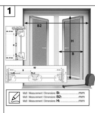
Determine clearance width measurement B, by measuring the horizontal inner distance to the open door. Determine clearance height measurement H, by measuring the vertical inner distance of the open door.
