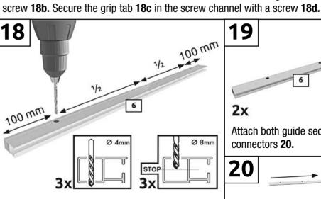
Drill through the guide section 6 three times with a 4 mm drill. When drilling, leave 100 mm distance to the ends of the individual guide sections and ensure the centre hole is equidistant between the two outer holes. Widen the holes on the front side of the sections using an 8 mm drill, so that the head of the screw fits through the hole.
