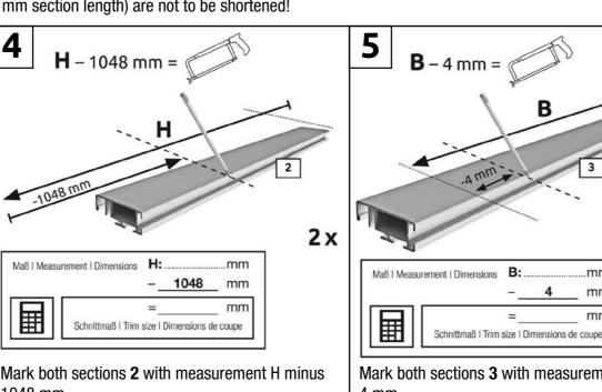
Mark both sections 3 with measurement B minus 1048 mm. **Example:** Measured clearance width B = 900 mm
