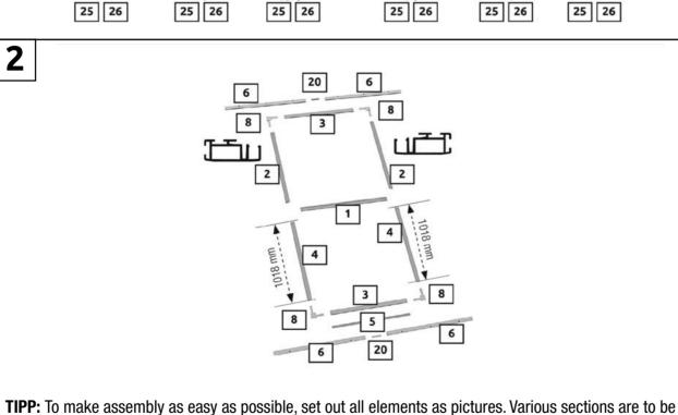
shortened according to the measurements of the following formulas. Both lower height sections 4 (1018 mm section length) are not to be shortened!
