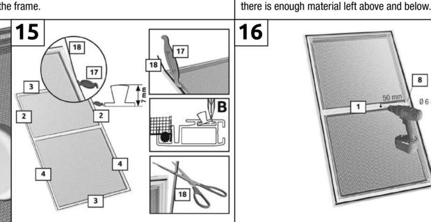
Place the 7 mm sealing brush 18 on the outer
