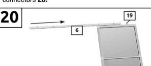
Push the connected guide sections 6 on the rollers **19** on the upper side of the door.
