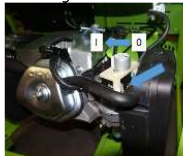
Throttle valve to position 0 for starting. To Pos. I during operation.
