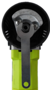
Figure 4: Place a wrench
