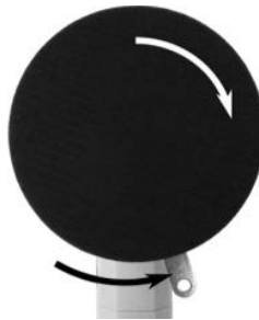
Figure 5: Screw the disc sanding pad on
