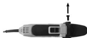
Figure 10: Remove the Allen screw
