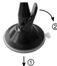
Figure 9 : Placer le support
