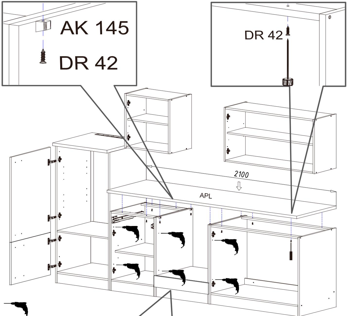
Mit  $\varnothing 5\text{mm}$  Bohrer durchbohren
